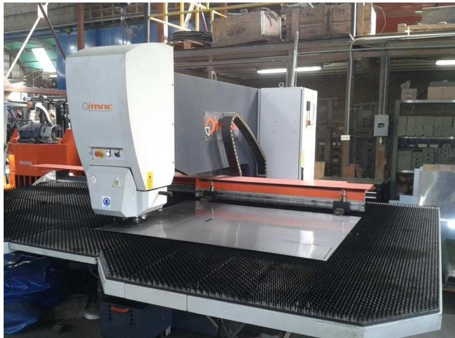
*Figura No. 8: Máquina Punzonadora CNC IMAC HP-1250 (3)*
