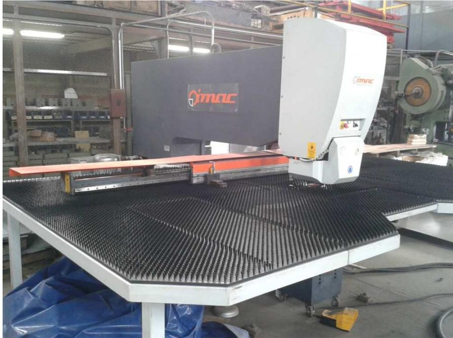
*Figura No. 7: Máquina Punzonadora CNC IMAC HP-1250 (2)*
